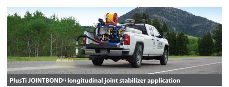
The PlusTi<sup>™</sup> family of smog-eating road penetrants includes JOINTBOND<sup>™</sup> superhydrophilic longitudinal joint stabilizer for asphalt pavements. Longitudinal joints and rumble strips in asphalt pavements are the most common and earliest point of pavement failure due to insufficient density during construction. Left unaddressed, these inherently weak joint areas reduce pavement life cycle by as much as 40 percent.
